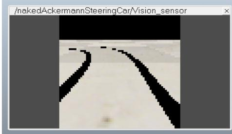
With this sensor, it is possible to obtain a two-dimensional image with a great range both near and far, observing both black lanes at all times.
